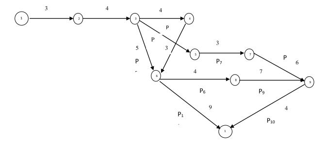
Fig I: Project Network of House Construction project
